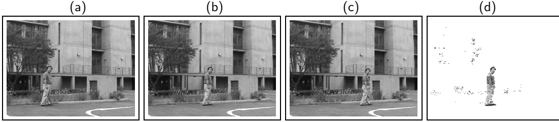
Figure 4: Motion detection from three successive images (a), (b) and (c) by using the Gaussian mixture model, the Markov random field model and the belief propagation. The result of motion detection is given in (d).
